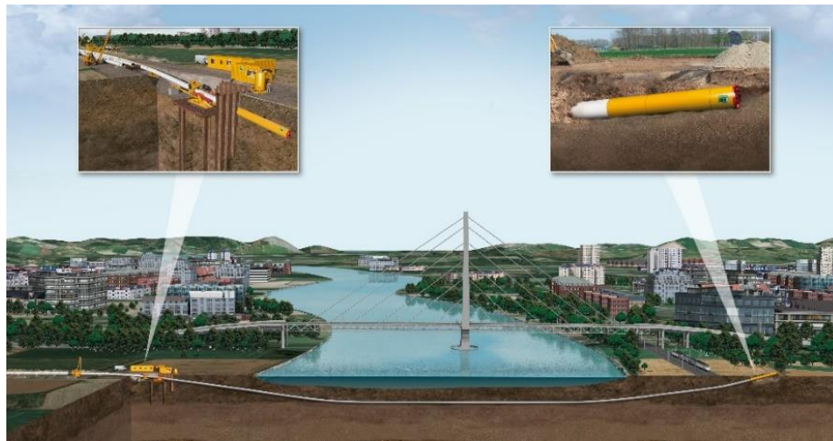
Figure 7. Functional principle of Direct Pipe for one-step pipeline installation
